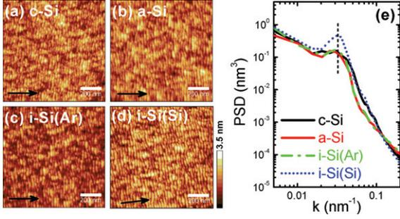
Fig. 1: (Colour on-line) (a)–(d) AFM images of nanoripples produced by IBS after 20 minutes of irradiation for the four different targets in table 1. The arrows show the direction of the Ar<sup>+</sup> beam. (e) Corresponding PSD of the morphologies.
