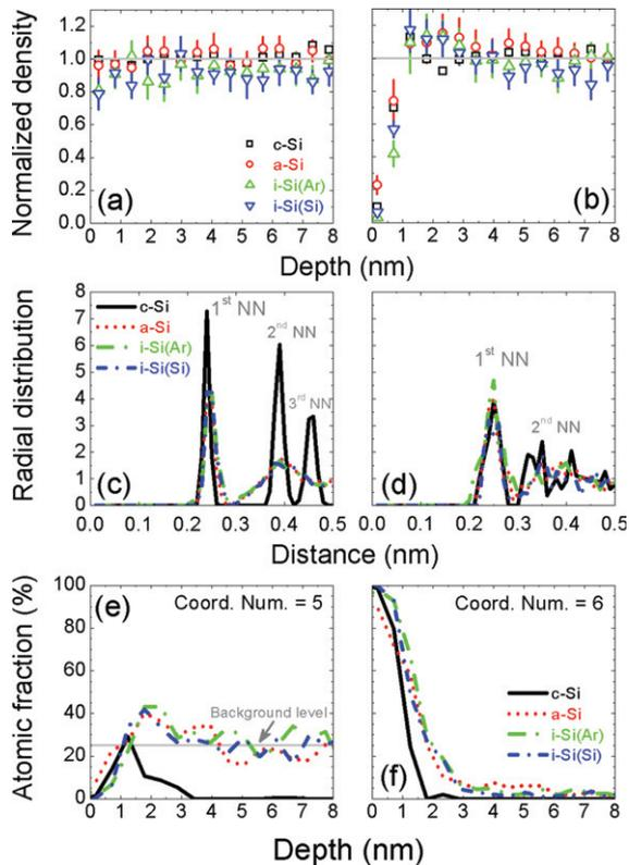
Fig. 3: (Colour on-line) Normalized atomic density ((a) and (b)) and radial distribution function ((c) and (d)) before and after 1000 Ar<sup>+</sup> impacts, respectively. Atomic fraction of Si atoms with coordination number equal to 5 (e) and 6 (f) after 1000 Ar<sup>+</sup> impacts.
