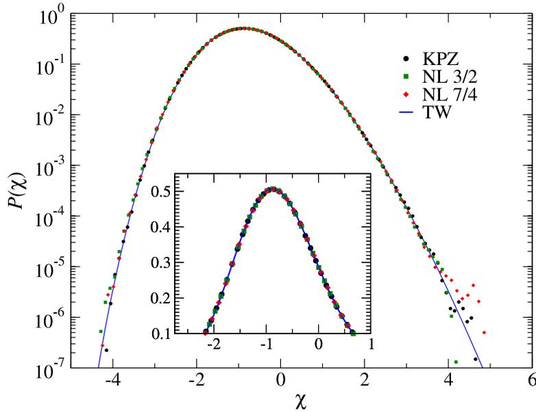
**Figure 3.** 1D height distributions for equation (1) (●) and equation (2) for  $\mu = 3/2$  (■) and  $\mu = 7/4$  (◆). The variable  $\chi$  is defined in the text. The solid blue line is the TW (GOE) distribution expected for  $d = 1$  [42].  $P(\chi)$  is estimated from 2048 independent runs starting from a flat initial condition. Inset: zoom of main panel, in linear representation. All units are arbitrary.
