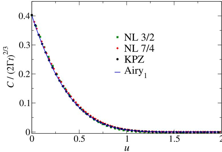
**Figure 4.** 1D height–height correlation function for equation (1) (●) and equation (2) for  $\mu = 3/2$  (■) and  $\mu = 7/4$  (◆). Here,  $u = x\sqrt{\Gamma/2\lambda}/(2\Gamma t^*)^{2/3}$  while  $C(x, t = t^*)$  is measured from the same surfaces employed to estimate  $P(\chi)$  in figure 3. The solid blue line provides the covariance of the  $\text{Airy}_1$  process [43]. All units are arbitrary.
